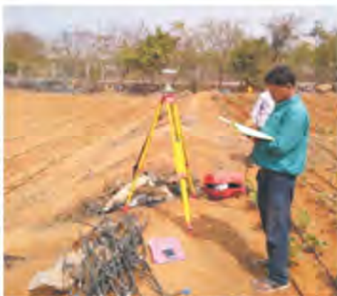
Ground Control Points (GCPs)
