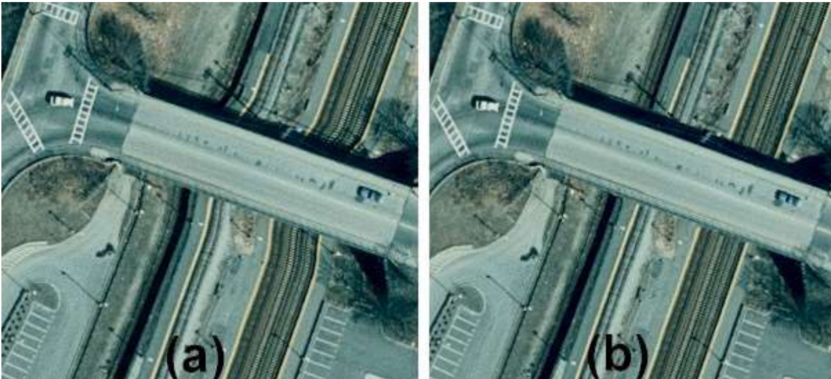
Figure 3. Figure shows local distortion over a bridge overpass with the distortion being eliminated after image editing
